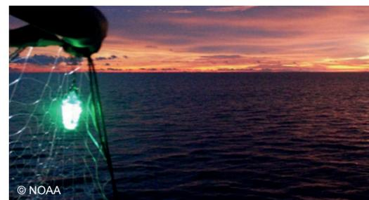
*LEDs can be attached to a fishing net to prevent bycatch of marine animals.*
